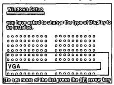
Press ENTER key while VGA is highlighted. The screen will return to previous Windows Setup screen, then check that Display setting was changed to VGA.
